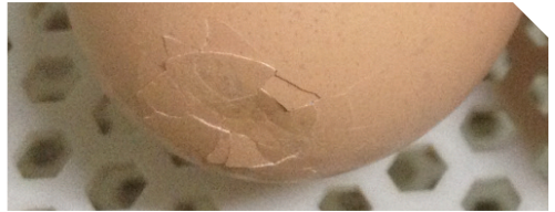
Figure 2 Excessive vacuum pressure on the egg lifter has caused damage to the blunt end of the egg.
