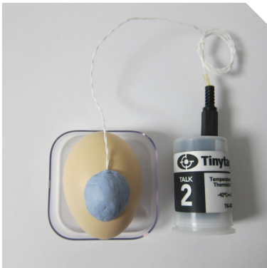
Picture 1 The Tinytag thermistor probe attached just below the equator of the egg with a thumb-nail sized lump of Blu-Tack.
