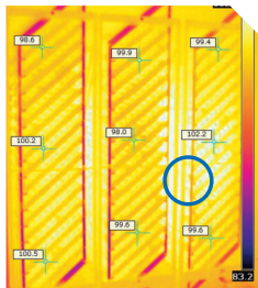
Figure 2 Hot area in a single stage setter.
