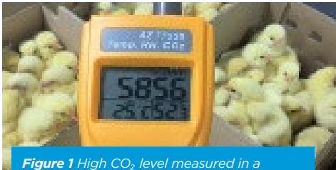
Figure 1 High CO 2 level measured in a holding room with insufficient ventilation.
