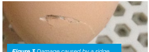
Figure 3 Damage caused by a ridge or bar on the handling equipment.
