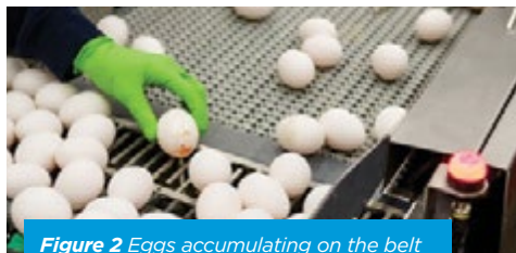
Figure 2 Eggs accumulating on the belt will have increased numbers of cracks.
