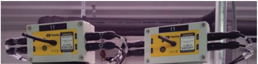
Figure 1 Radio controllers for TinyTags allow real time measurement of egg shell temperature (EST) in operating setters.
